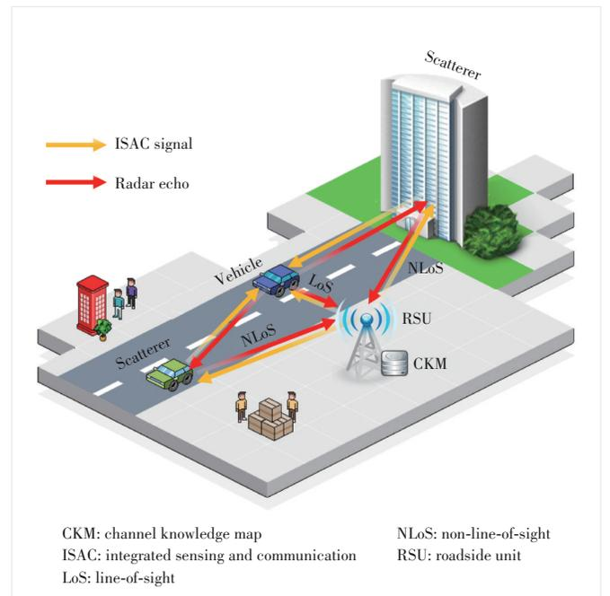
▲ Figure 3. Considered scenario of CKM-assisted ISAC beam tracking system
