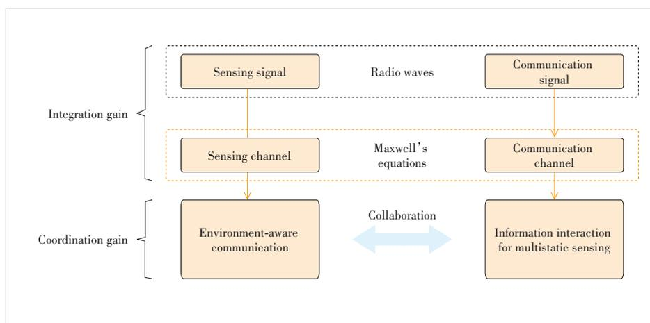
▲ Figure 1. Two main advantages of integrated sensing and communication (ISAC): integration gain and coordination gain
