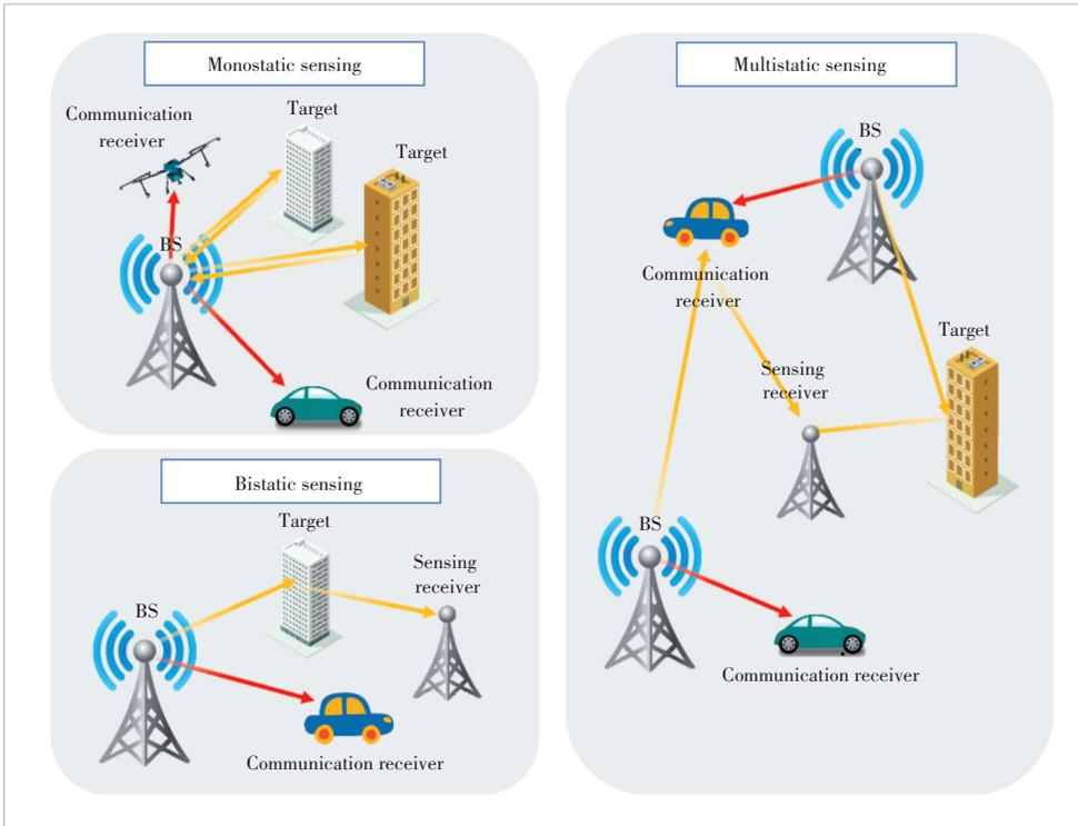
▲ Figure 2. Typical integrated sensing and communication (ISAC) systems, where the sensing target can be the communication receiver itself in all the scenarios
